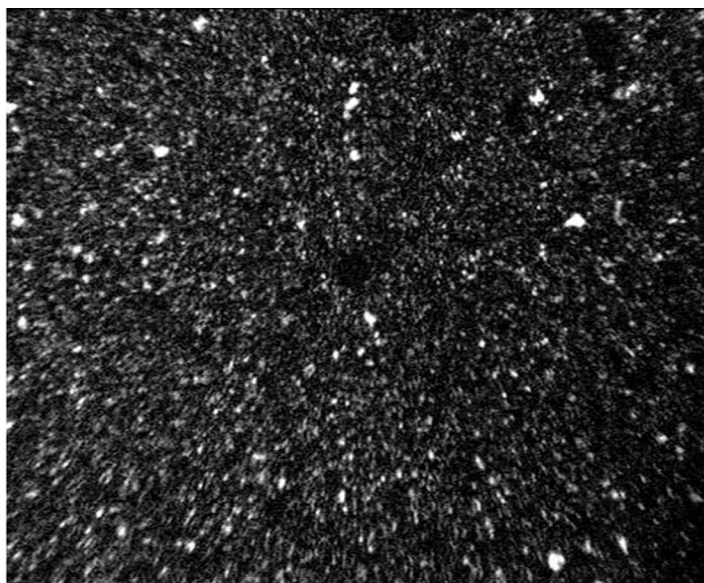
Figure 3. The birefringence texture micrograph of the ligand, MPTPP, at 25°C.
